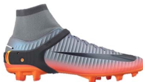
Figure 2. The PlayerMaker™ system fitted to the ankle of the right foot. The complete system includes an identically sized and fitted inertial measurement unit for the left ankle.
